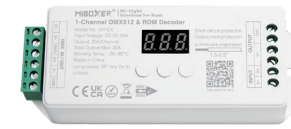
D1-CX 1-Channel Constant Voltage DMX & RDM Decoder
