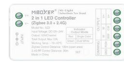
SZ2 2 in 1 LED Controller (Single Color / Dual White)
